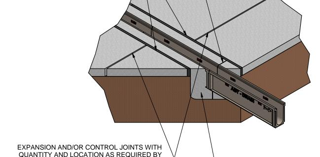
CHANNEL ENCAPSULATION CONCRETE THICKNESS, STRENGTH, AND REINFORCEMENT AS DETERMINED BY-STRUCTURAL ENGINEER AS SUITABLE FOR APPLICATION
